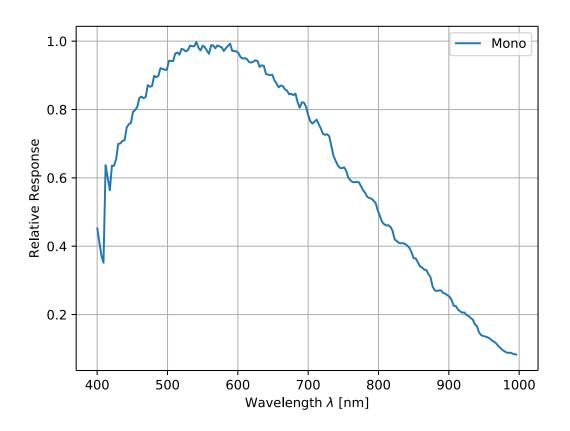
The spectral response curve excludes lens characteristics.
