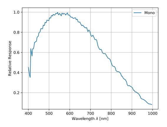
The spectral response curve excludes lens characteristics.
