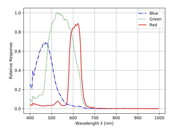
The spectral response curve includes IR cut filter characteristics, but excludes lens characteristics and light source characteristics.
