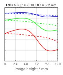
— 20 LP/mm, radial 40 LP/mm, radial — 80 LP/mm, radial --- 20 LP/mm, tangential --- 40 LP/mm, tangential --- 80 LP/mm, tangential
