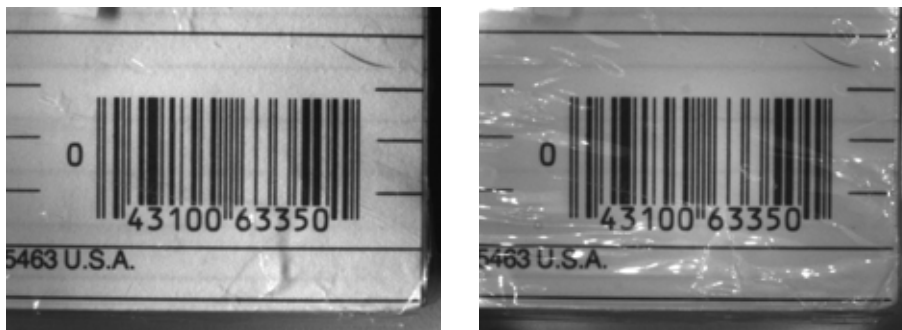
Fig. 1 - Cellophane wrapper on a pack of note cards. Left: meets all 3 Acceptance Criteria. Right: meets only criteria 1 & 2. In this circumstance, the “wrinkle” is not precluding a good barcode reading, but what if the “wrinkles” were in a different place in the next pack on the line?
