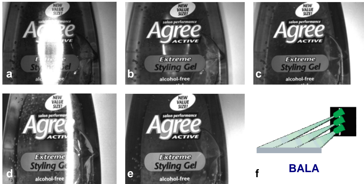
Fig. 15 - A change in lighting – sample – camera geometry or type may be more effective than applying polarizers to stop glare. a – Coaxial Ring Light w/o Polarizers. b – Coaxial Ring Light w/ Polarizers (note some residual glare). c – Off-axis Ring Light w/o Polarizers. d – Off-axis Linear Array Light (BALA) oriented parallel to the bottle long axis. e – Off-axis Linear Array Light oriented perpendicular to bottle long axis. f – BALA light function diagram.
