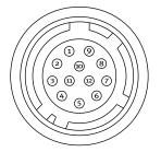
Camera side: Equivalent to Hirose Electronic HR-10A-10R-12PB(72) Cable side: Equivalent to Hirose Electronic HR10A-10P-12S(73)
