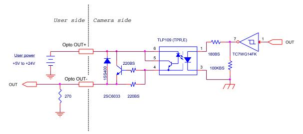
Characteristics of the recommended circuits for Opto OUT
