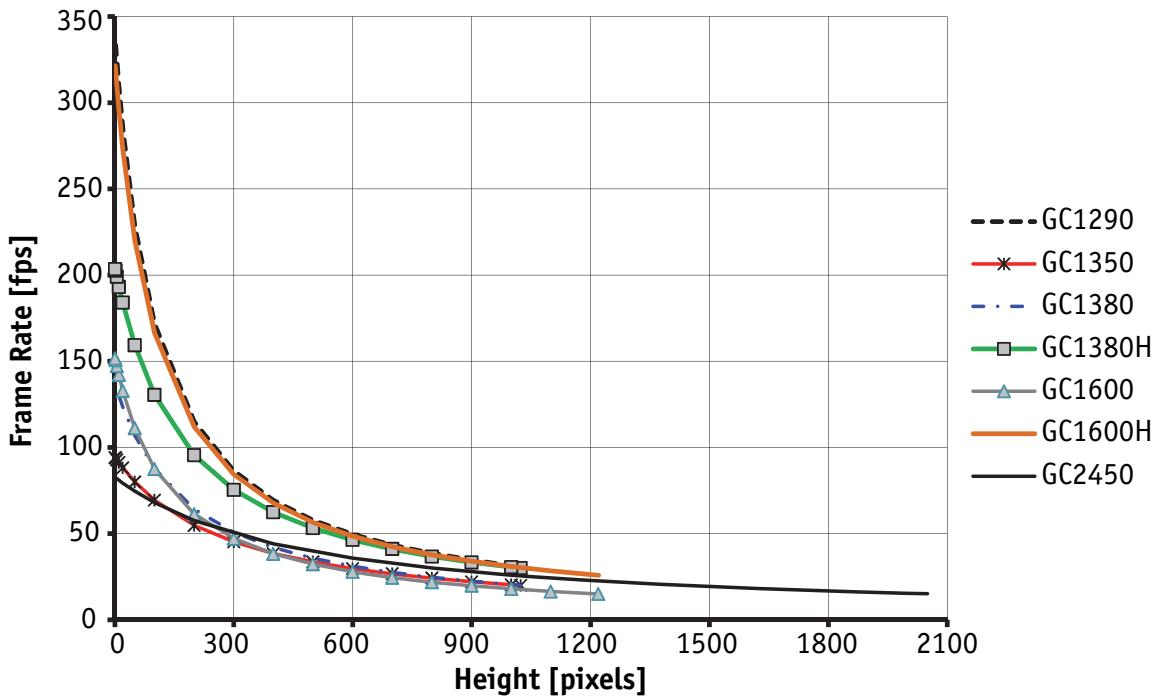
Figure 55: Maximum frame rate comparison for select models
