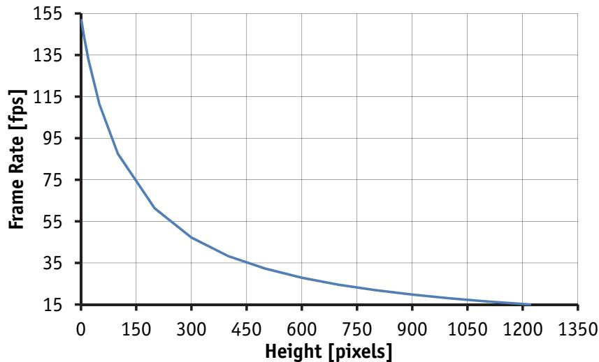
Figure 51: Frame rate vs. height for Prosilica GC1600
