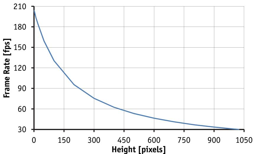
Figure 50: Frame rate vs. height for Prosilica GC1380H
