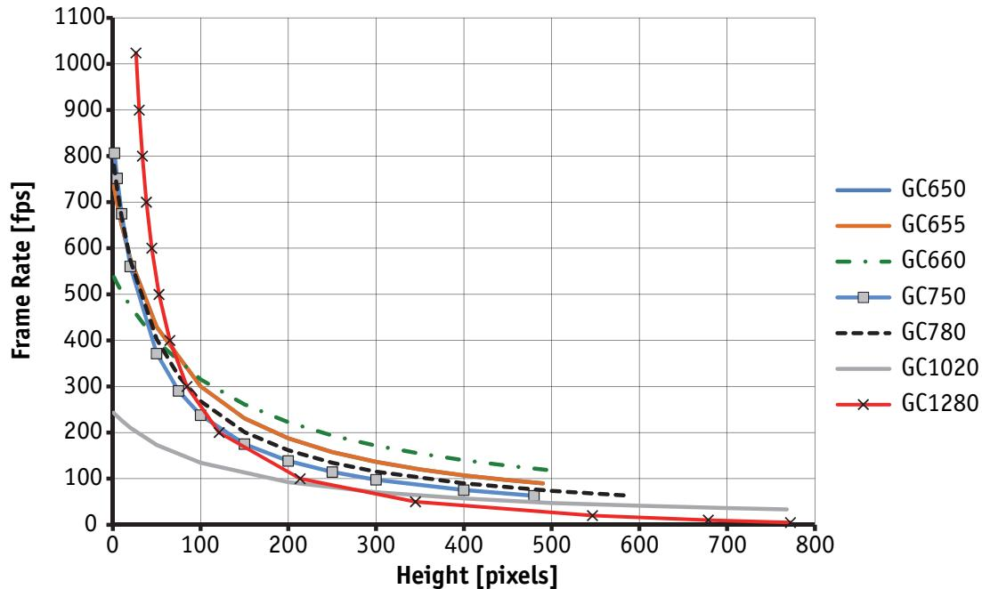
Figure 54: Maximum frame rate comparison for select models
