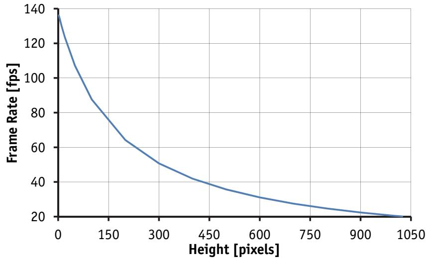
Figure 49: Frame rate vs. height for Prosilica GC1380
