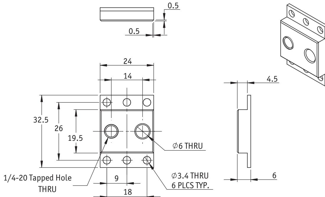
Figure 31: Prosilica GC tripod mount mechanical drawing
