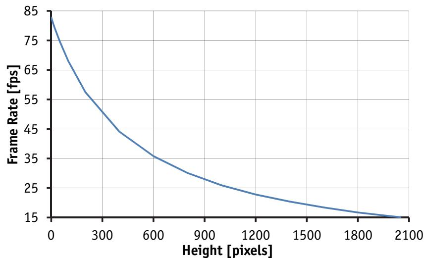
Figure 53: Frame rate vs. height for Prosilica GC2450
