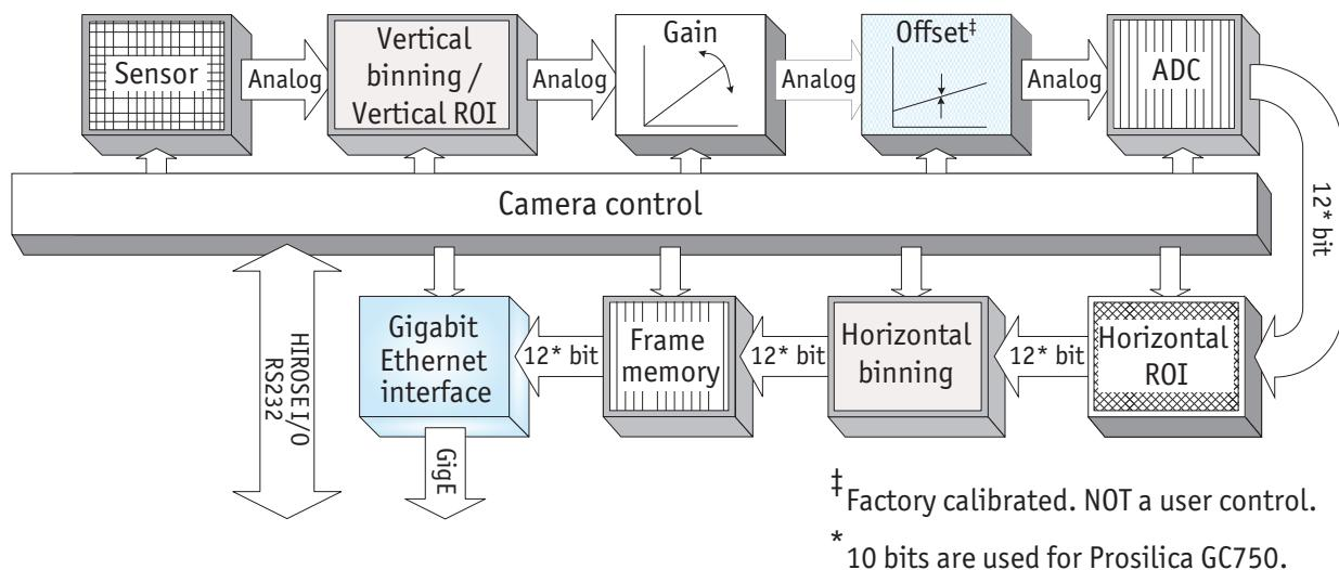
Figure 56: Block diagram of monochrome Prosilica GC cameras
