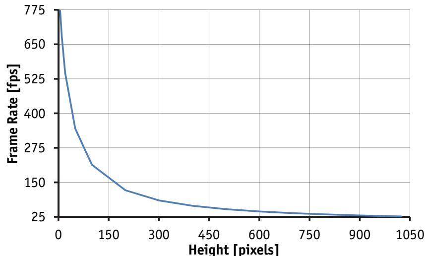
Figure 46: Frame rate vs. height for Prosilica GC1280
