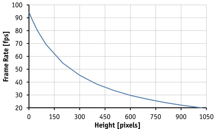
Figure 48: Frame rate vs. height for Prosilica GC1350
