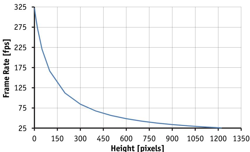
Figure 52: Frame rate vs. height for Prosilica GC1600H
