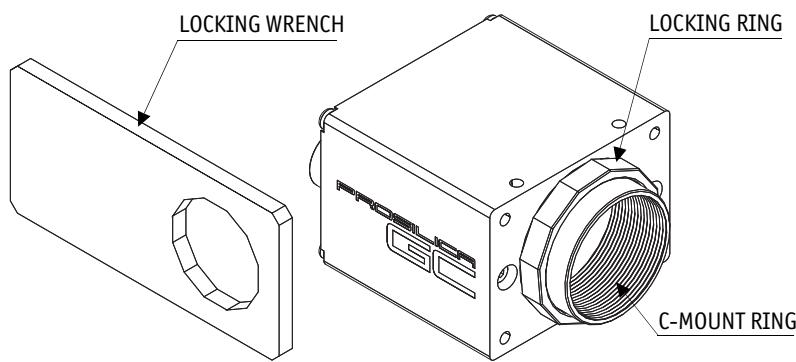
Figure 33: Prosilica GC camera and locking wrench
