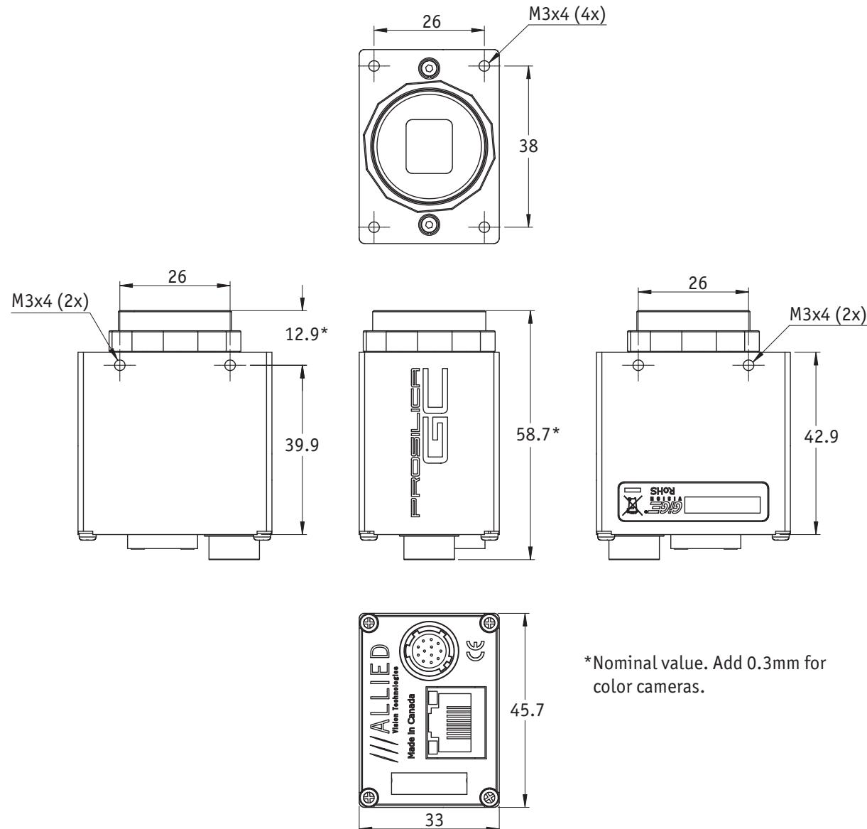
Figure 30: Prosilica GC CCD models mechanical dimensions
