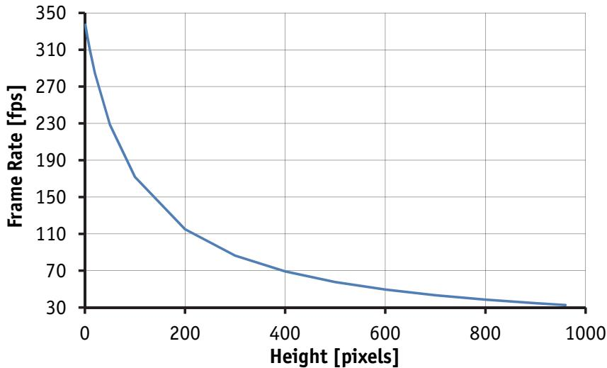
Figure 47: Frame rate vs. height for Prosilica GC1290
