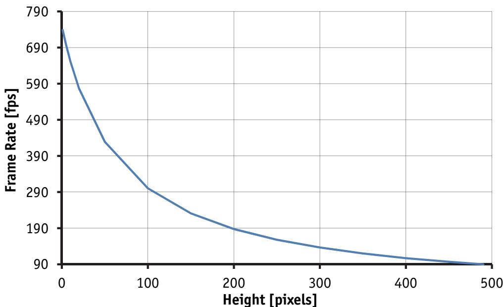
Figure 40: Frame rate vs. height for Prosilica GC650
