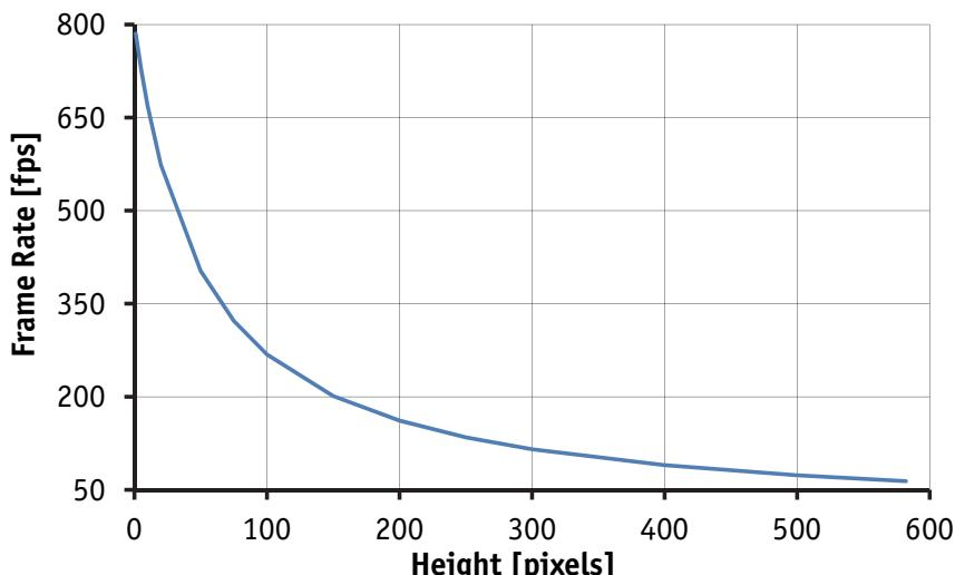
Figure 44: Frame rate vs. height for Prosilica GC780
