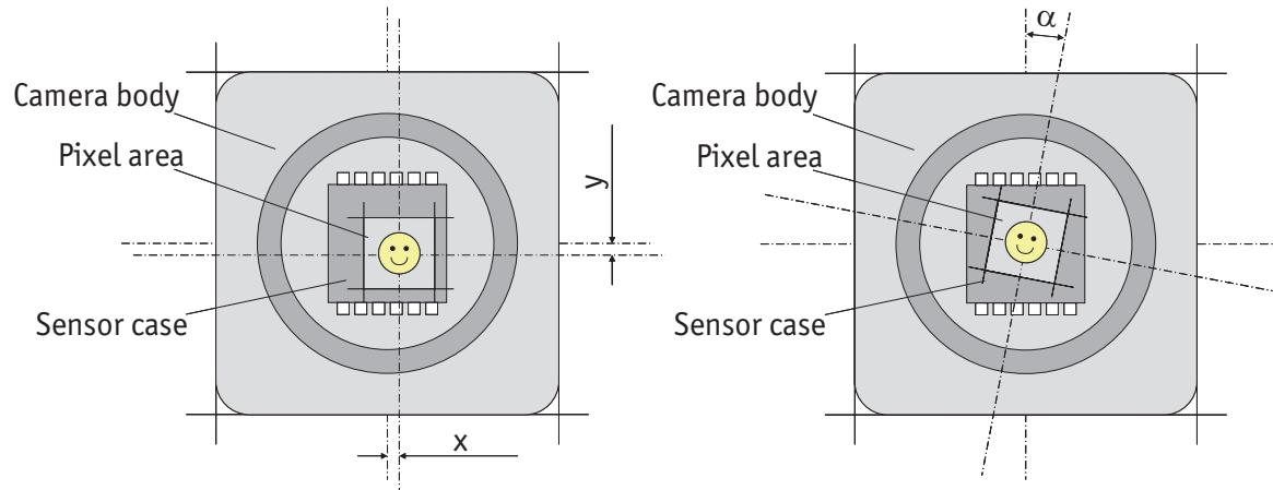
**Method of Positioning:** Video alignment of photo sensitive sensor area into camera front module. (lens mount front flange)
