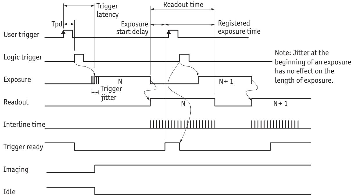
Figure 39: Prosilica GC internal signal timing waveforms
