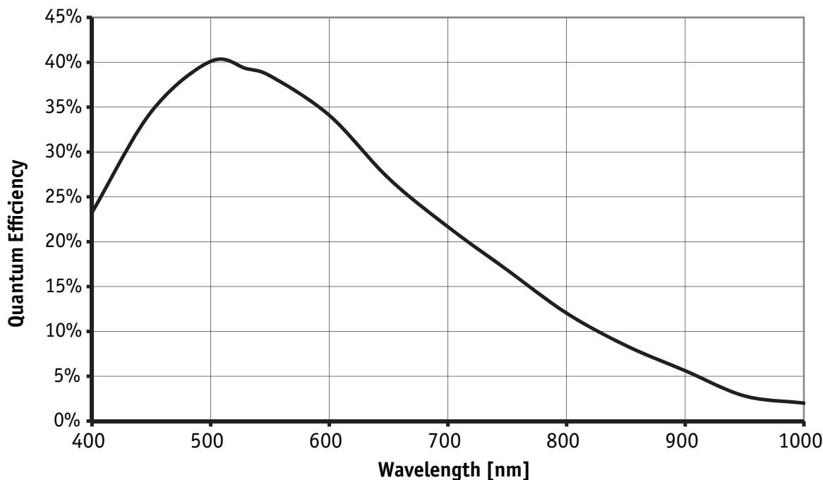
Figure 9: Prosilica GC780 monochrome spectral response
