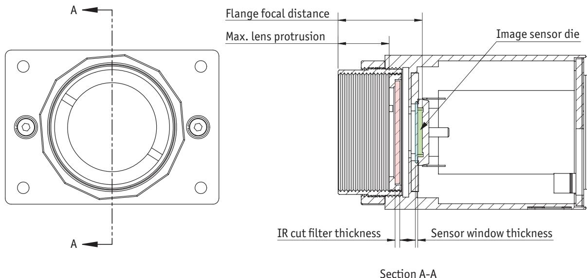
Figure 32: Cross section of typical Prosilica GC assembly with C-Mount
