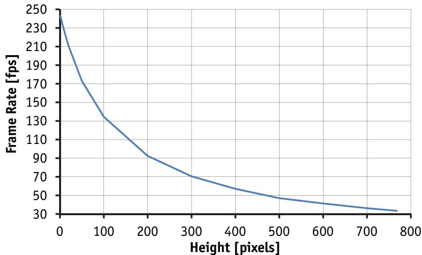
Figure 45: Frame rate vs. height for Prosilica GC1020
