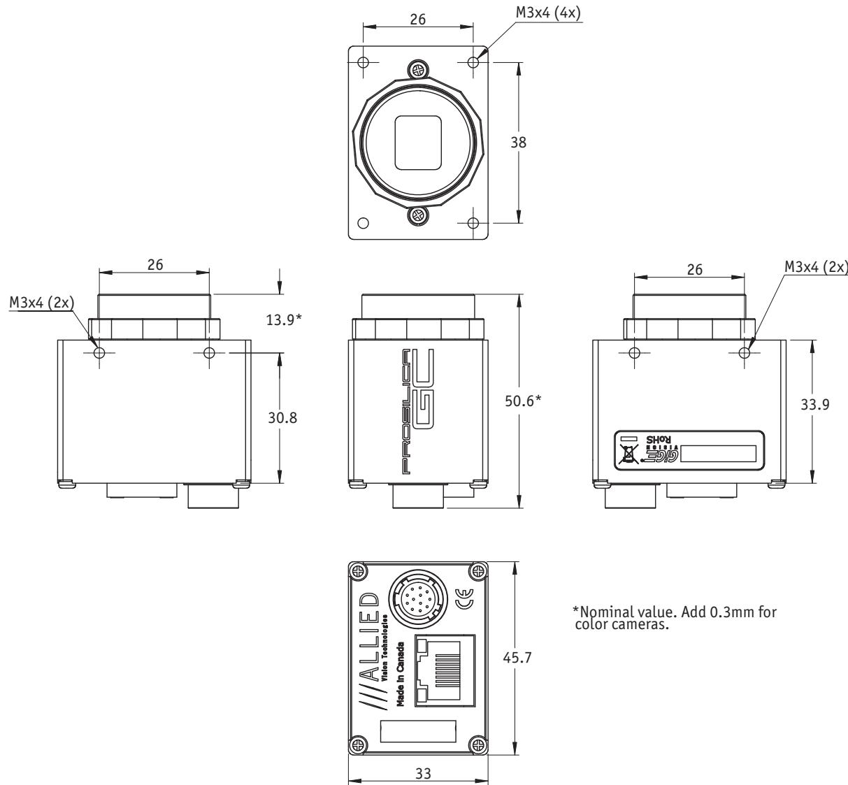
Figure 29: Mechanical dimensions for Prosilica GC750, and GC1280
