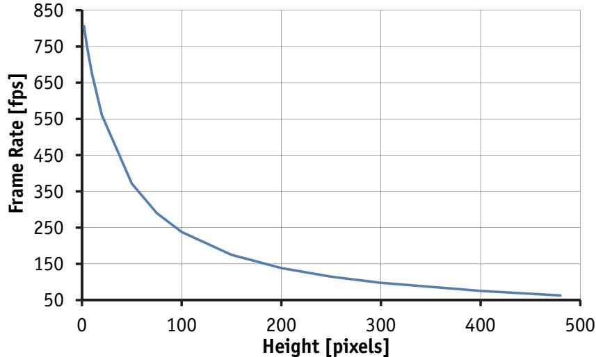
Figure 43: Frame rate vs. height for Prosilica GC750
