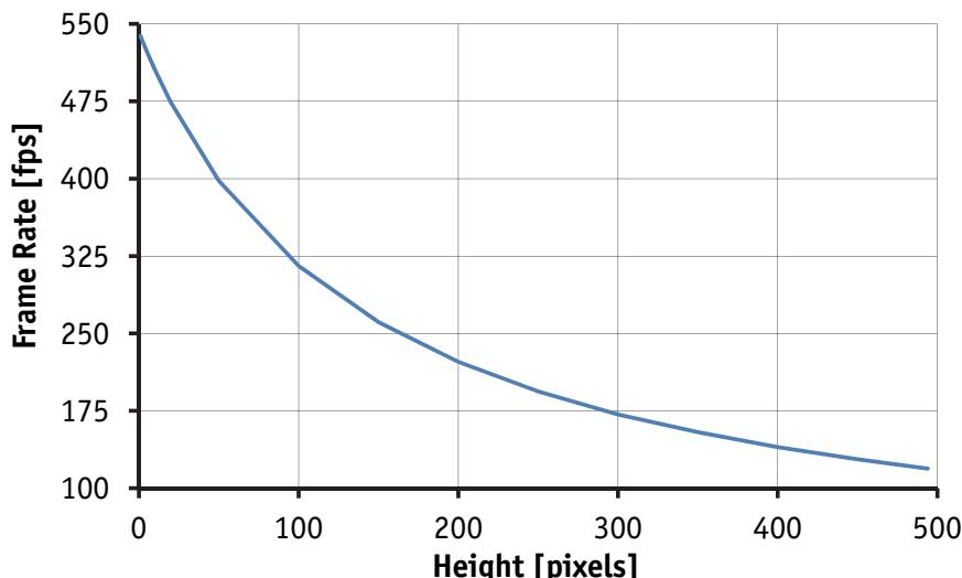
Figure 42: Frame rate vs. height for Prosilica GC660
