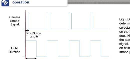
Light Duration is determined by the selectable set time on the PTM and does NOT depend the camera strobe signal. Light triggers on rising edge of strobe pulse.
