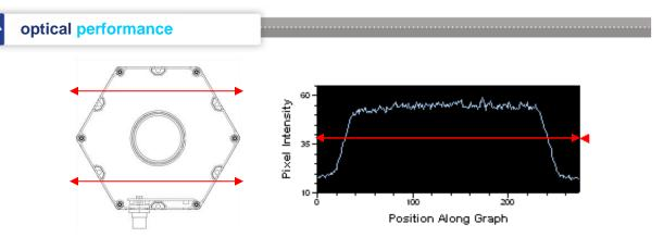
The ODRD130 offers a very diffuse light pattern at a defined working distance between 150mm – 450mm. The Pixel Graph representation shows a steep drop off in intensity outside of the active area with a very diffuse light pattern inside.
