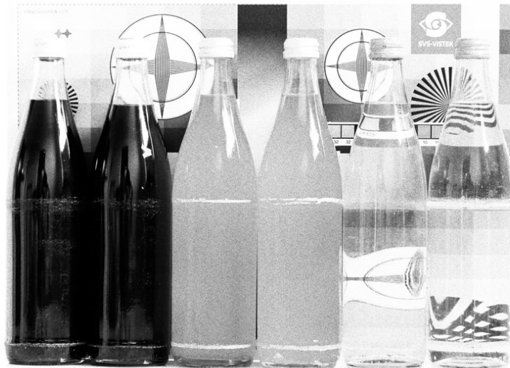
noise caused by too much gain
