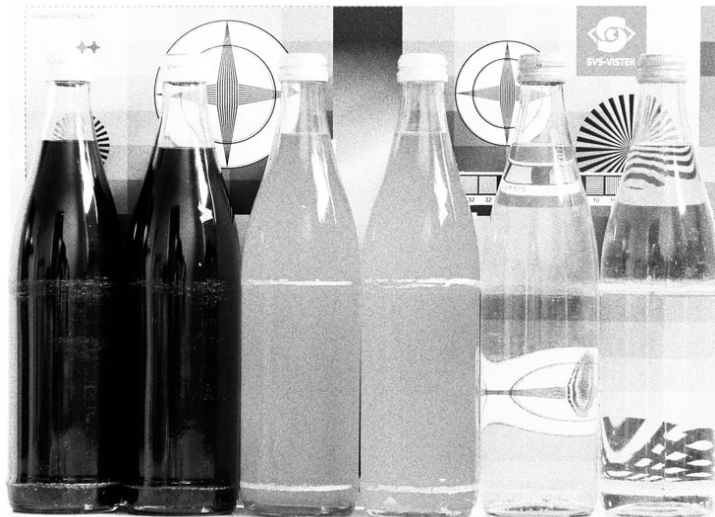
noise caused by too much gain
