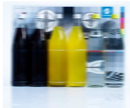
Figure 3: moving object, global shutter
