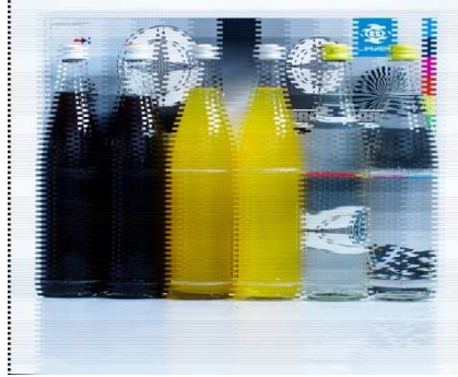
Figure 5: moving object, interlaced camera
