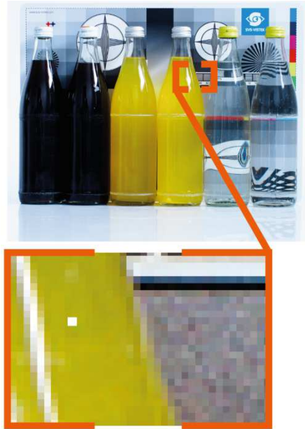
Figure 17: Illustration of a defect pixel
