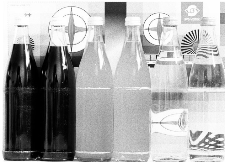
noise caused by too much gain
