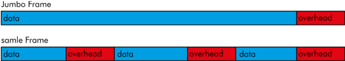
Figure 5: Illustration of data reduction with jumbo frames
