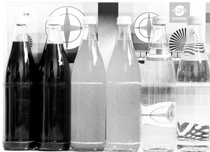
Figure 26: noise caused by too much gain
