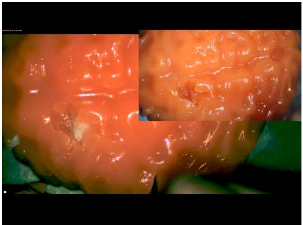
VIDEO 2: Modeled brain tumor in a brain phantom made of Gelatin
