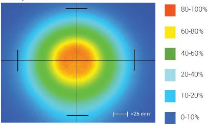
Optical measurement taken using SL112-WHI @ 300 mm
